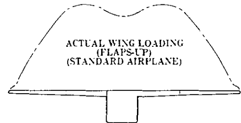
Figure 5 — Actual wing loading — flaps up.
