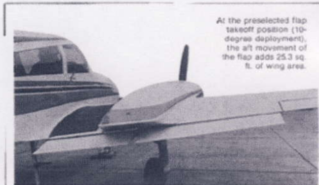
During cruise the Robertson Fowler-action flaps tuck neatly under the wing.
